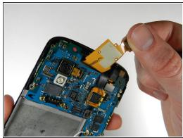
Gently pry the metal tab up using a spudger, and lift up the disconnected black flap.
