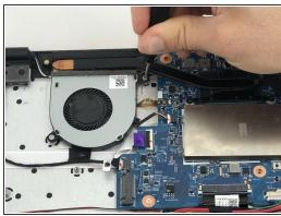
Use Phillips #1 screwdriver to remove the two 4mm screws that are securing the fan.
