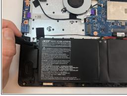
Use a Phillips #1 screwdriver to remove two 4 mm screws that secure the battery.
