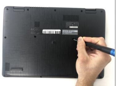
• Use a Phillips #1 screwdriver to remove the thirteen 6.5mm screws that secure the back cover.
