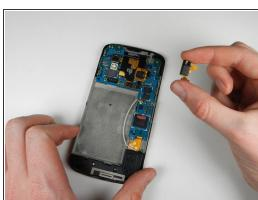
Gently lift the audio jack upwards and to the left to remove it from the motherboard.
