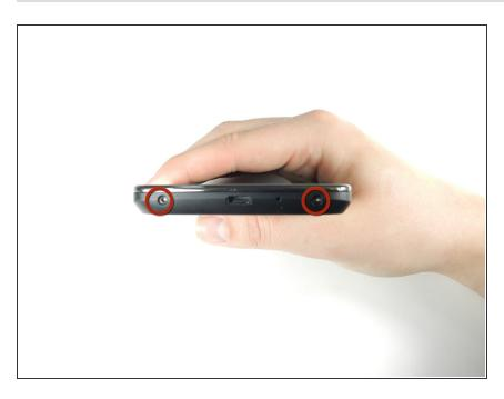
Remove the two screws from the bottom of the phone with a <u>T5 Torx</u> <u>Screwdriver</u>.
