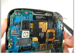
Using a spudger, pop off the gray connector on the top right of the motherboard.
