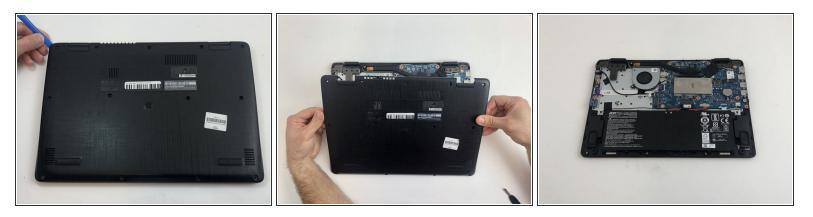
Use a plastic opening tool to gently separate the back cover from the laptop. A snapping sound will be heard as a signal that the clips are being disengaged.
