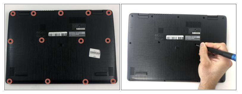
Use a Phillips #1 screwdriver to remove the thirteen 6.5mm screws that secure the back cover.
