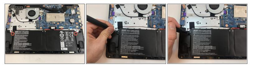
• Use a Phillips #1 screwdriver to remove two 4 mm screws that secure the battery.
