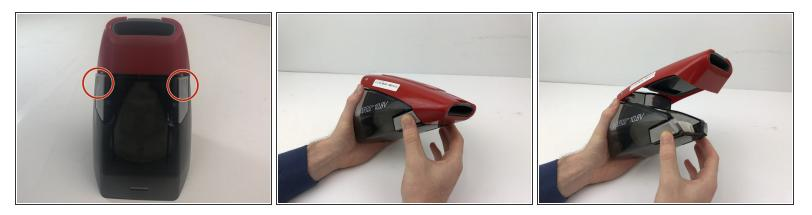
• Press the two grey buttons on either side of the filter chamber inwards to release the chamber.
