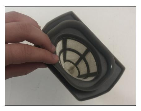
Replace it with a new or restored filter by placing it back in the filter chamber.
