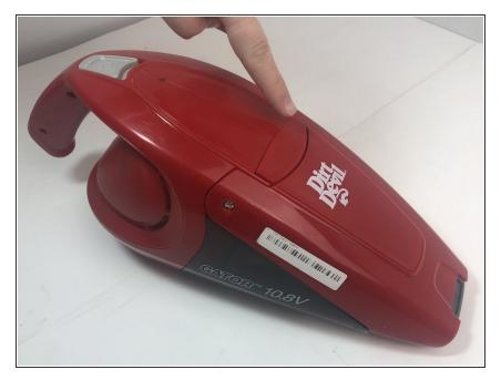
To get to the filter, press the button on the top of the vacuum to split your device in two.
