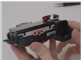
Remove four M1.5x4mm screws using a PH00 Phillips screwdriver.
