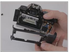
Once the screws have been removed, unsnap and lift the rear plastic cover off of the camera.
