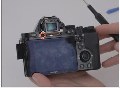
Remove the four M 1.5x2mm screws.
