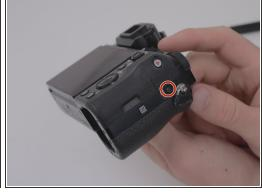
Remove the six M1.5x4mm screws with a PH00 Phillips screwdriver.
