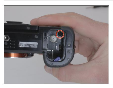
Remove one M1.5x4mm screw with a PH00 Phillips screwdriver.
