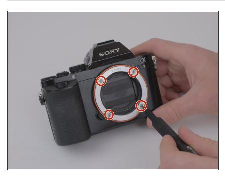
Remove each of the four M1.5x4mm screws with a PH00 Phillips screwdriver.
