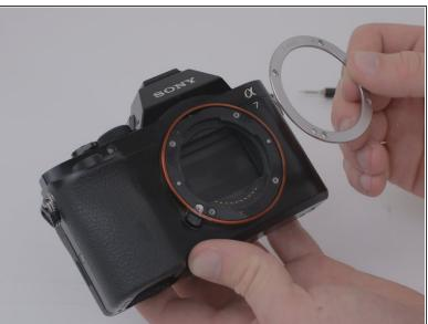
• Lift the circular, metallic plate out of the base of the lens assembly, and set it aside.
