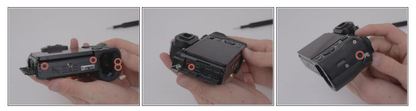
• Remove the six M1.5x4mm screws with a PH00 Phillips screwdriver.
