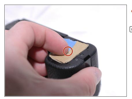
Slide the switch over to the right side to open the battery door.
