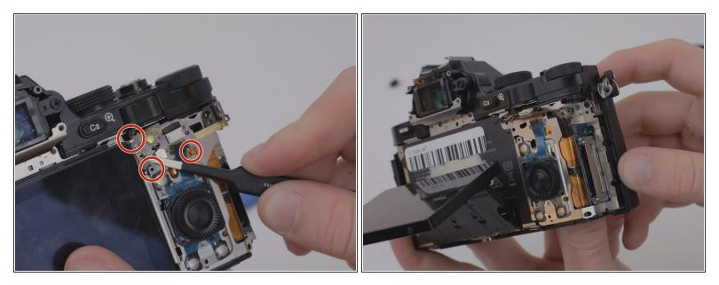
Place the tweezers on the side of the circuit board and lift it from underneath so as to free it from the three retaining tabs.
