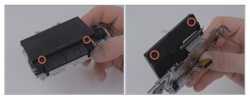
• Remove four M1.5x2mm screws with a PH00 Phillips screwdriver.
