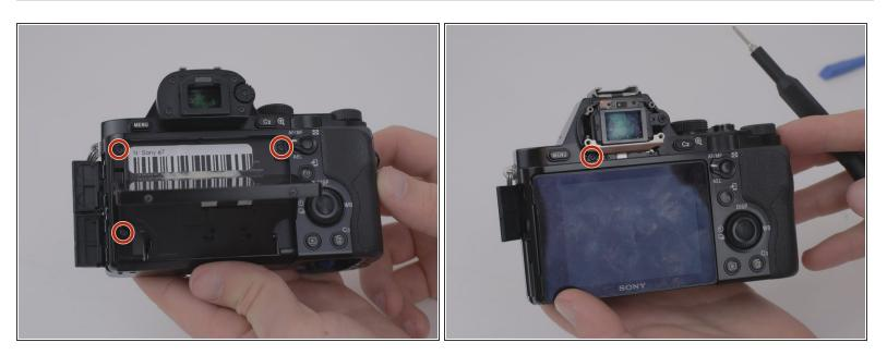
• Remove the four M 1.5x2mm screws.
