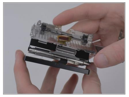
• Seperate LCD screen from its metal backing.
