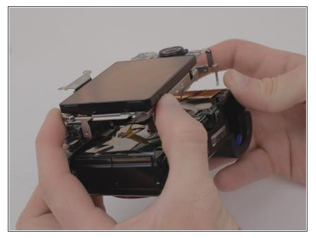
• Lift the metal plate and LCD screen away from the camera body.
