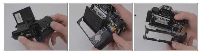
• Once the screws have been removed, unsnap and lift the rear plastic cover off of the camera.
