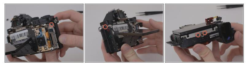
• Remove four M1.5x4mm screws using a PH00 Phillips screwdriver.
