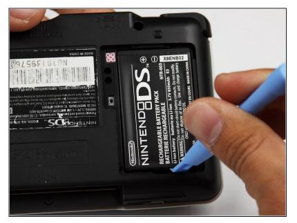
• Use a plastic opening tool or spudger to pry out the battery from the bottom. If a plastic opening tool or spudger isn't available, your fingernails may work.
