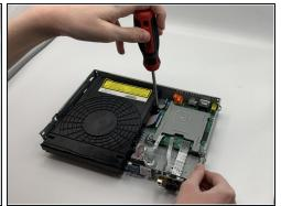
• Remove the two Phillips #1 screws using a screwdriver.
