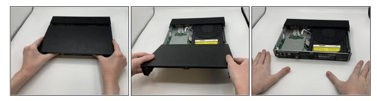
Remove the top cover by sliding it off.
