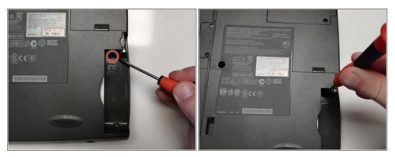
• Remove the single 4mm Torx screw, located beneath the floppy disk drive bay.
