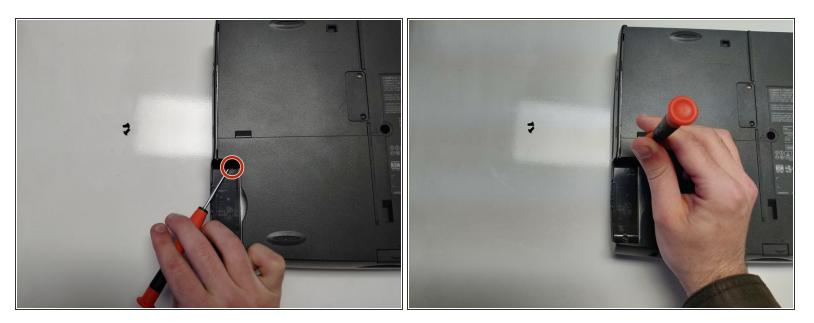
• Remove the single 4mm Torx screw from beneath the battery pack bay.
