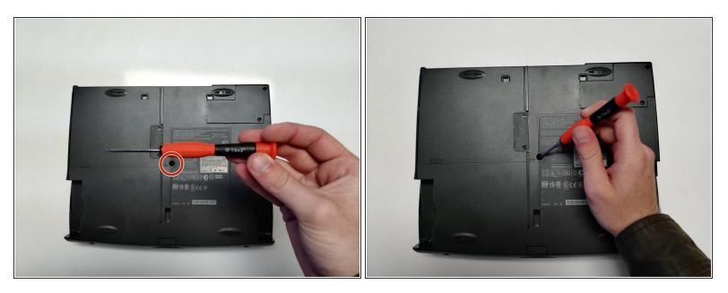
• Remove the single 4mm Torx screw from the bottom center of the laptop.
