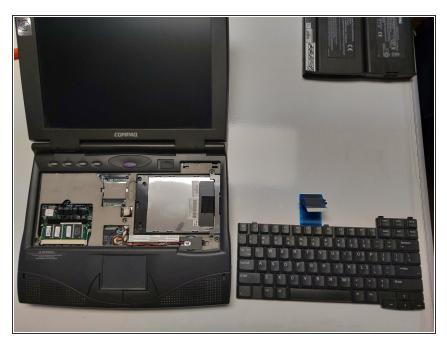
• Completely remove the keyboard.
