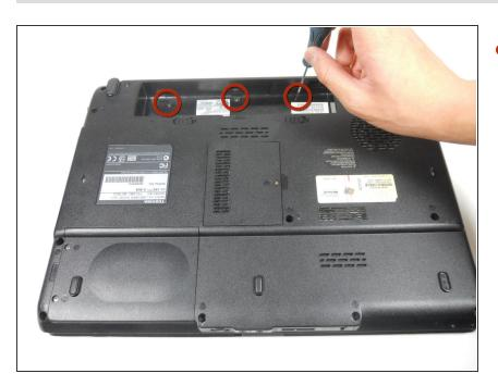
Remove the three 3.7 mm type-00 Phillips head screws located in the battery compartment.
