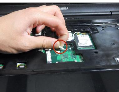
Using your fingers, remove the white plastic connector located to the right of the ribbon connector.
