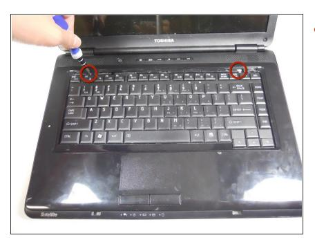
Remove the two 4.8 mm screws from underneath the plastic cover piece using a Phillips #00 screwdriver.
