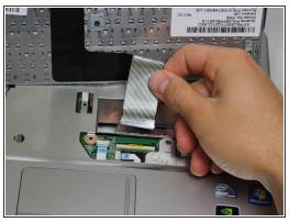
• Carefully pull the ribbon cable connecting the keyboard and the laptop to remove from the device.
