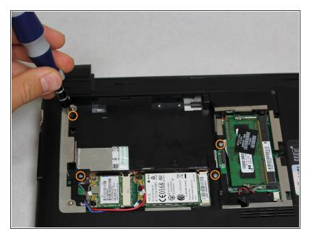
Unscrew the four Phillip 00 5.6 mm screws located around the wireless card and RAM.
