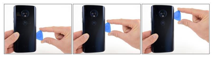
Slide the pick along the right edge of the rear glass to separate the adhesive underneath.
