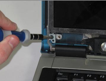
• Use the Phillips 00 screwdriver to remove the two 6.72mm screws at the bottom left and right of the screen.
