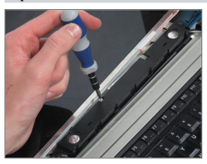
Use the Phillips 00 screwdriver to remove the 5.54mm screw connecting the green panel to the laptop frame.
