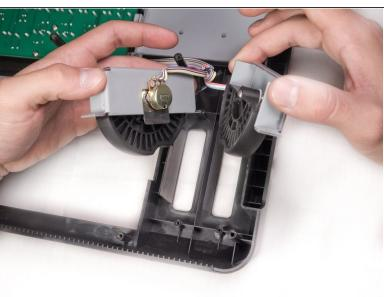
Using a Phillips #2 screwdriver, remove the four 9.5 mm silver screws holding the knobs to the face plate.
