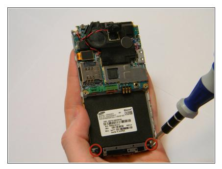
Remove the two 4.0 mm screws, one silver and one black, from both ends of the antenna using the Phillips 00 screwdriver.
