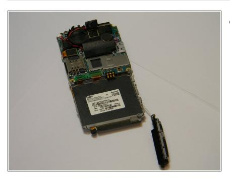
To remove the antenna, disconnect the white antenna cable that connects it to the main circuit board.
