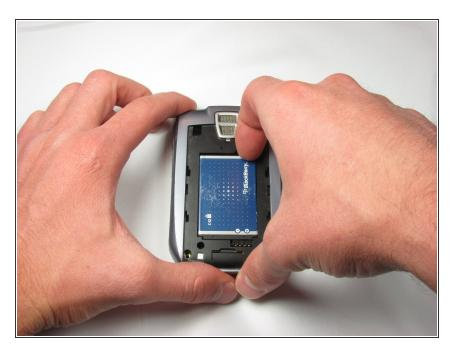
To remove the battery, place your fingernail in the slot at the top right of the battery and pull up.
