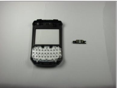
Next, use a metal spudger to unhook the earpiece from the inside of the front panel.
