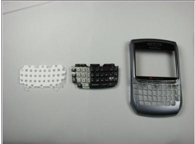
When the front face plate has been pulled away, be sure to grab the keypad as it may fall out.
