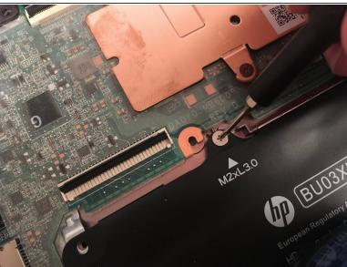
Remove the four 3mm Phillips #000 screws holding the battery in place.
