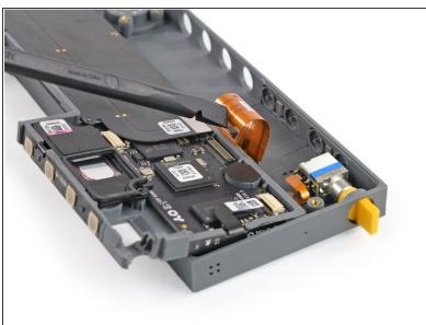
Use the flat end of a spudger to disconnect the flex cable from the front panel assembly.
