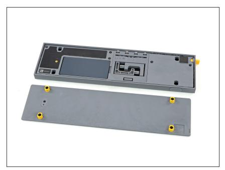
Remove the bottom plate including the rubber feet.
