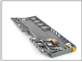
Flip the midframe over to gain access to the flex cable connector underneath.
