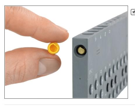
For reassembly align the flat side of the knob with the flat side of the axle.
