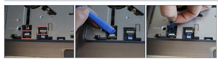
Use the opening tool to unplug the palm rest cables and slide the cables out.
