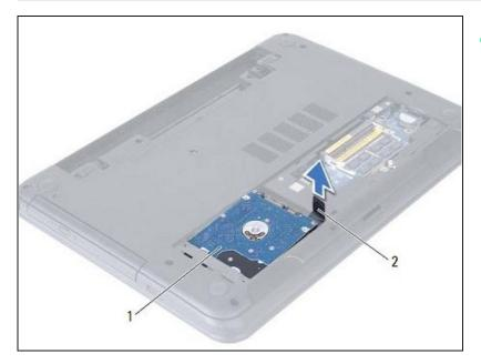
Slide the hard-drive assembly backward to connect the harddrive assembly to the system board.
