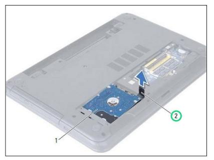
Using the pull-tab, lift the harddrive assembly out of the computer base.
