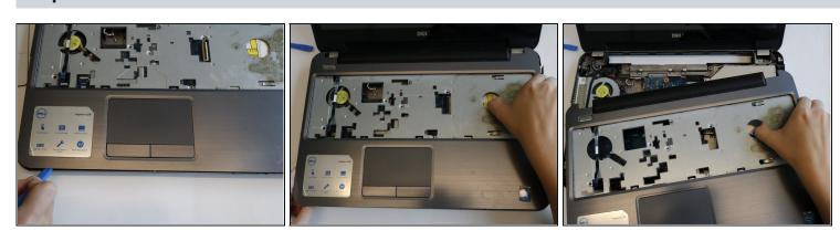
Use the opening tool to lift the edges of the palm rest. Once all of the sides are lifted, pull the palm rest off.
