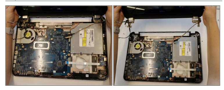
Remove the display assembly by lifting the display from the hinges.
