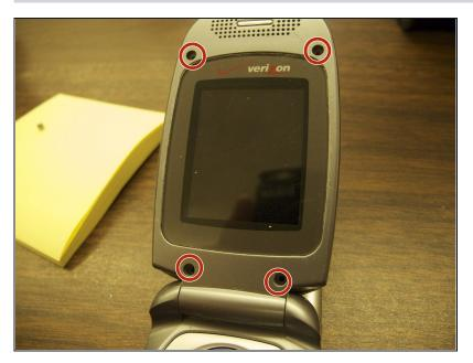
Using the Phillips screwdriver, carefully remove all four screws.
