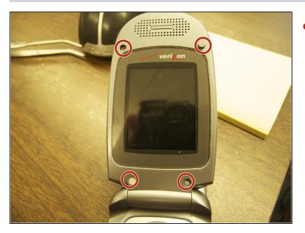
• Remove the rubber stoppers from the four corners of the front screen.
