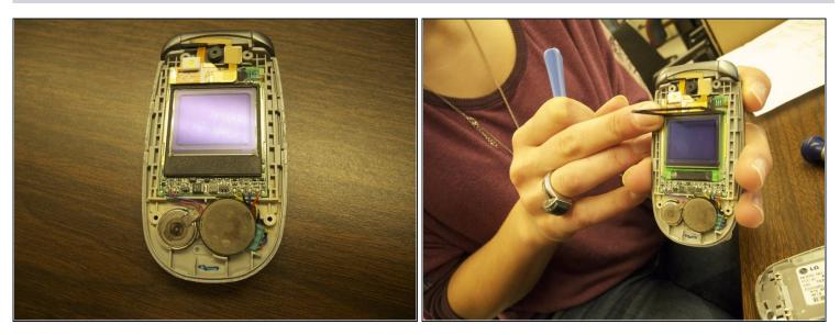
• Carefully lift off the black frame around the LCD screen and set it aside.
