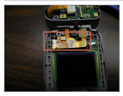
• Using tweezers, carefully disconnect the orange ribbon from the computer chip.
