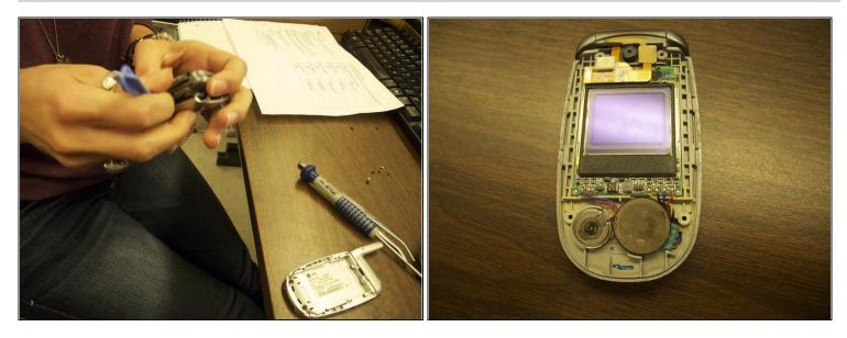
• To pry open the face plate, place the iFixit Opener tool in the crease of the phone.
