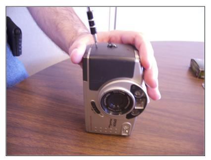
Remove 2 screws on the rounded side of the camera wisdom here.
