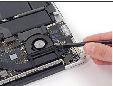
Move the antenna cables aside, clear of the AirPort board.
