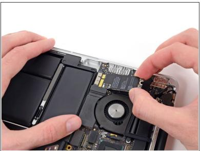
Pull the AirPort board straight out of its socket on the I/O board.
