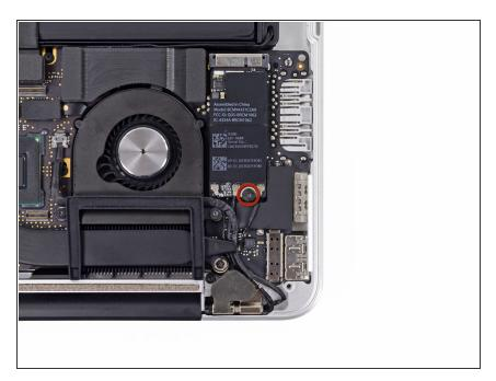
Remove the single 2.7 mm T5 Torx screw securing the AirPort board to the I/O board.
