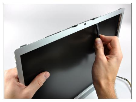
• Work your way along the top edge of the LCD, slowly prying the attached steel strip away from the front bezel.
