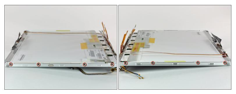
• Remove the four 3 mm Phillips screws from each side of the display (eight screws total).
