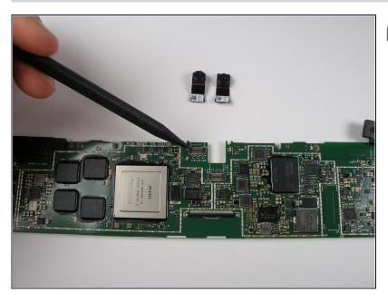
When you replace the camera(s), and make sure that they line up with the front and back cover.
