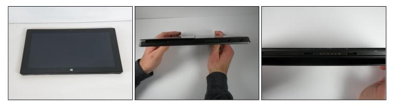
Prior to any repairs make sure that the device is orientated correctly, and you are familiar with all ports and buttons. The screen should be facing up with the Windows logo located on the bottom.
