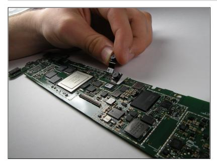
• Avoid touching the lens of the camera and unplug it from the bottom of the motherboard.
