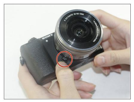
Place the camera in front so the lens is facing you. There should be a small button on the bottom left side of the lens.
