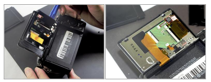
• Carefully open the back plate of the screen.
