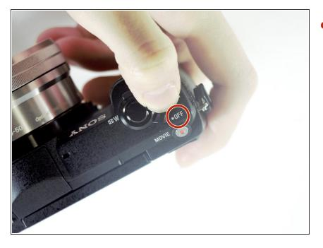
Slide the power switch on the top of the camera to "off."
