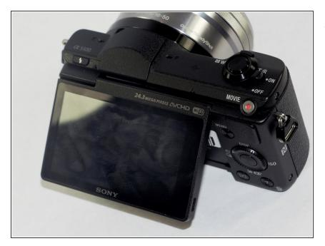
Flip the LCD screen so that you have access to the back of the screen. The front of the screen should be facing the direction that the lens is facing.
