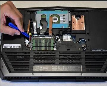
• Use the iFixit opening tool to disconnect the battery cable. Put the iFixit tool underneath the cable and then pull it to remove.
