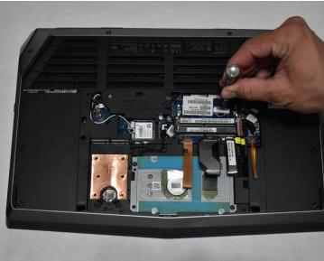
Using a Phillips #0 remove the small 1X 3mm screw behind where the RAM used to be.
