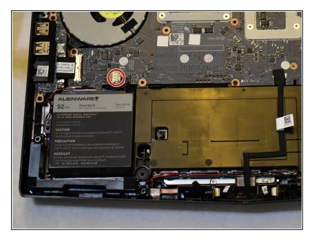
Remove the red, white, blue, and black colored wires connected to the motherboard.
