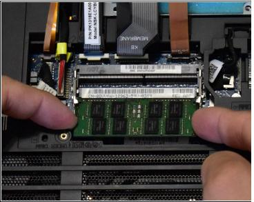
• Find the RAM located near the edge of the computer closest to you. Locate the small latches on either side of the RAM stick and push in the two latches to release. Gently grasp the RAM stick on either side and pull straight out. Repeat for the second RAM stick.
