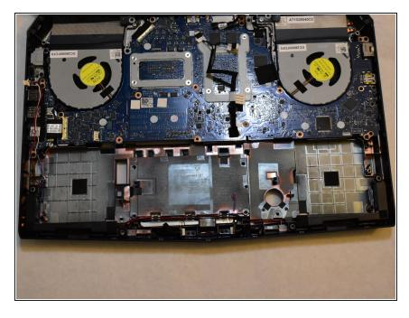
Lift the battery from the front edge and remove.
