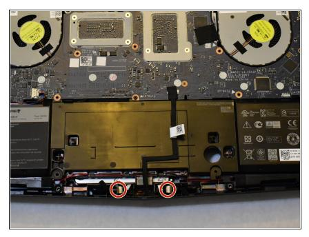
Disconnect and move aside the left and right wires.
