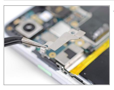
Remove the button array connector bracket.
