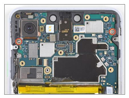
Remove the two 3 mm long T3 screws securing the motherboard.
