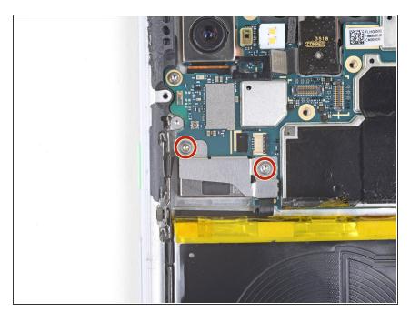
Remove the two 3 mm long T3 screws securing the button array connector bracket.
