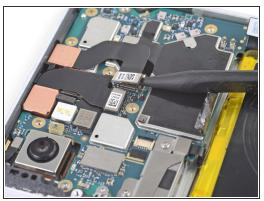
Use the point of a spudger to carefully pry up and disconnect the cameras from their motherboard sockets.
