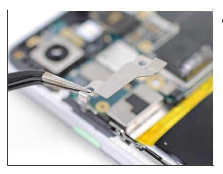
Remove the button array connector bracket.
