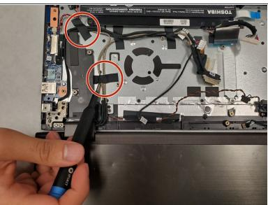
Remove all of the black tape securing the hinge to the laptop.
