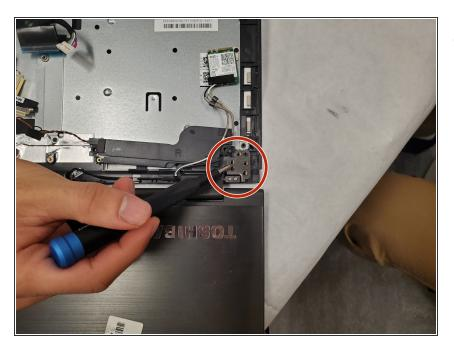
Repeat the previous step to remove the screws on the other hinge securing the display to the device.
