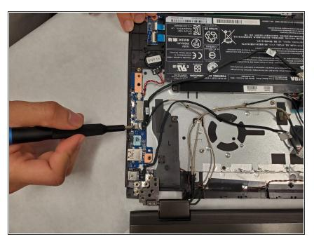
Disconnect the connector directly above the IO cable.
