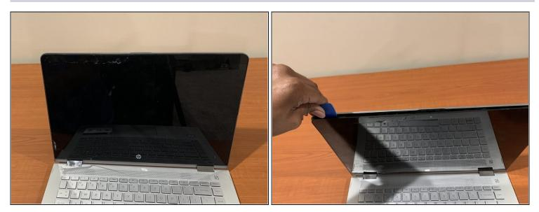
• Insert an opening pick between the screen and top case to separate it from the laptop.
