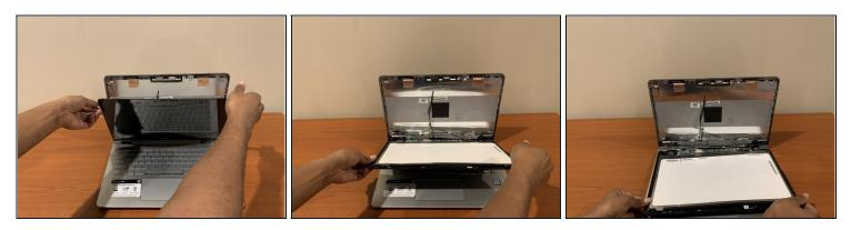
• Once the screen is pryed away from the laptop, lay the screen face down onto the keyboard.
