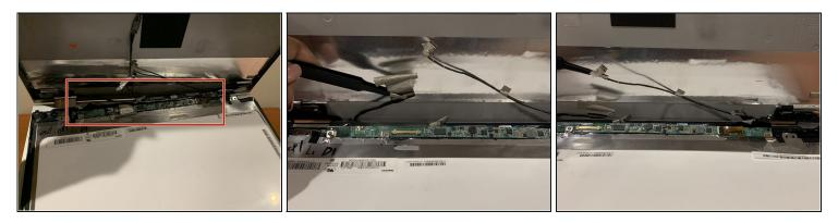
• Remove any tape or wires that connect the screen and laptop together using tweezers.
