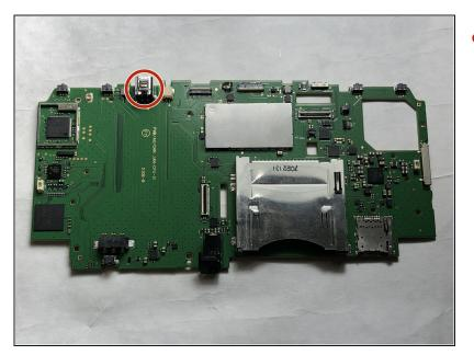
Remove the motherboard and locate the charging port. Flip the the motherboard over.
