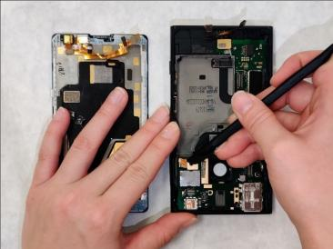
Disconnect the two gold connectors from the motherboard using a spudger.
