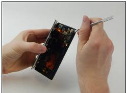
Wedge a spudger underneath the silver rectangle in the upper right corner until it pops off the back of the phone.
