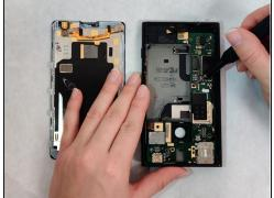
• Using a T4 screwdriver, remove four 4.60 mm screws to disconnect the motherboard from the rest of the device.
