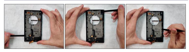
• Insert the spudger on the edges of the base and lift up.
