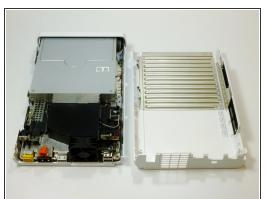
• On the back of the console, lift up and release the main top cover.
