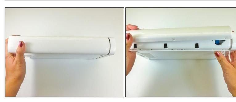
On the side opposite of the exhaust vents, slide the cover faceplate towards the back of the console and pull upwards to release it.
