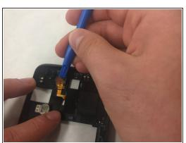
Peel off the orange cable using a plastic opening tool.
