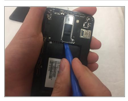
Pry off the silver button housing using the plastic opening tool.
