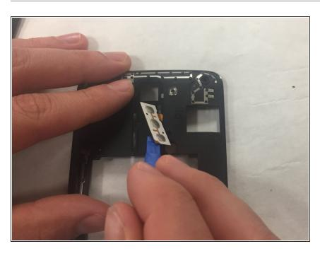
Remove the volume/power button cable from the rest of the phone using the plastic opening tool to break the adhesive.
