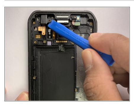
Use a plastic opening tool to pry the headphone jack up, and remove the headphone jack from the rear case. To reassemble your device, follow these instructions in reverse order.
