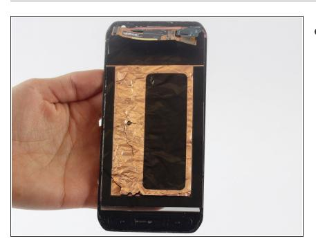
Remove the display assembly (LCD and Digitizer).
