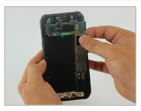
Remove the motherboard from the rear case.
