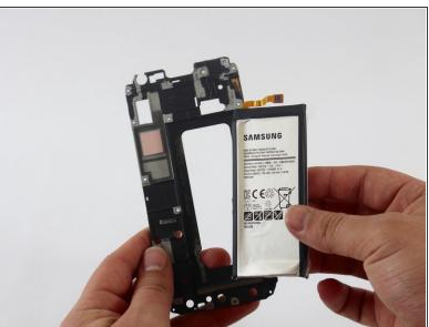
Remove the battery from the frame.
