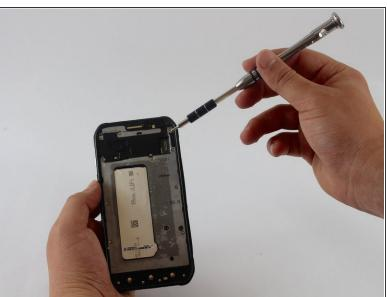
Use the Phillips Head Screwdriver sized PH000 to remove the sixteen 4mm screws from the frame.
