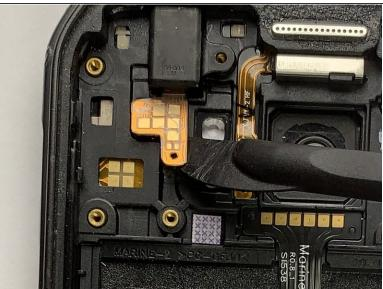
• Insert a spudger at the bottom, between the headphone jack connection and the rear case, to loosen the headphone jack.
