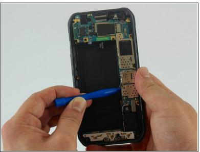
Insert the flats end of the spudger below the motherboard and twist it to pry the board up.
