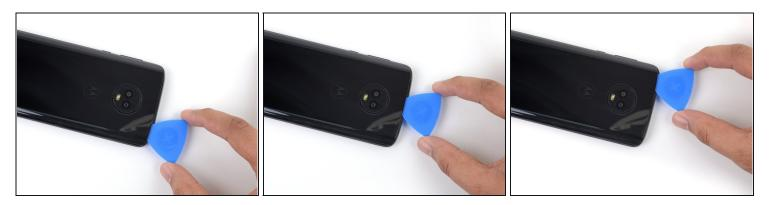
• Slide the pick all along the top edge of the phone to slice through the adhesive securing the rear glass.
