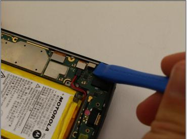
• Using the iFixit opening tool, pop up the three press-fit connectors in the bottom right corner of the motherboard.
