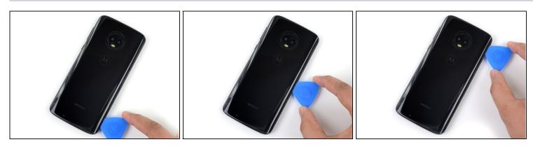
• Slide the pick along the right edge of the rear glass to separate the adhesive underneath.
