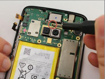
• Remove the two black 2.7 mm screws from the motherboard.
