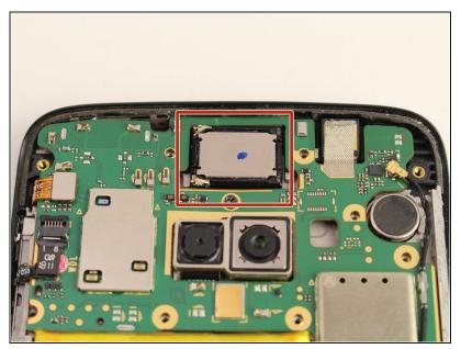
With the interior plate removed, locate the speaker.
