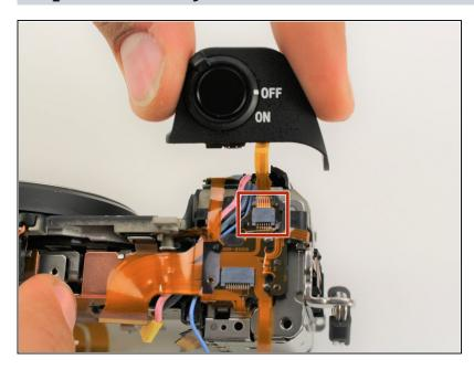
• Unplug the small ribbon located underneath the ON/OFF button and detach the button assembly from the camera.
