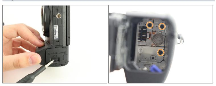
• Flip the battery lock switch to open and open the battery compartment.
