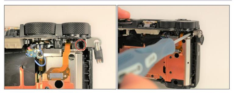
• Use the long, thin, screwdriver to remove one 5 mm JIS 00 screw inside the camera accessible below the dials from the back.
