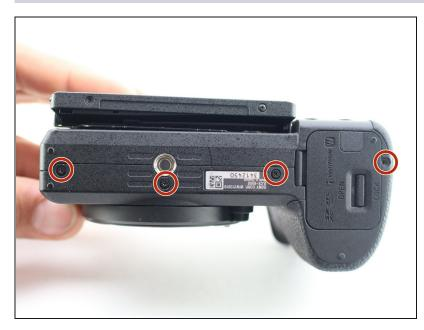
• Remove four 4 mm JIS 0 screws from the bottom of the camera.
