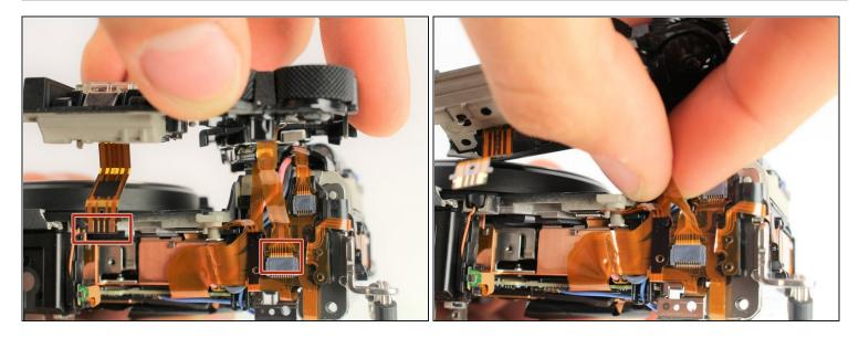
• Carefully unplug the two ribbon connectors attaching the top assembly to the rest of the camera.
