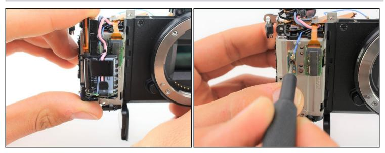
• Flip the black capacitor mount up and remove the 2.5mm JIS 00 screw located directly underneath it.
