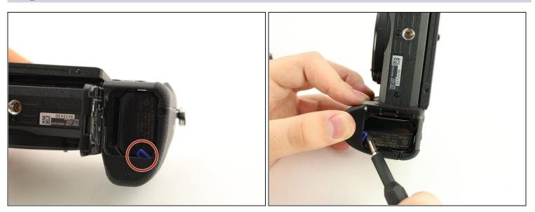
• Push the blue lever aside to release the battery.
