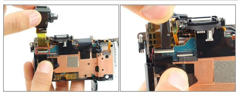
• Lift the viewfinder out and flip up the tab to release the wire ribbon where it is connected to the motherboard.
