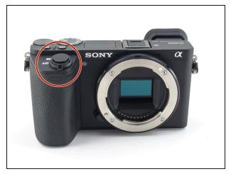
Verify the camera is powered off by setting the switch to OFF.
