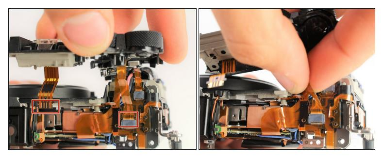
Carefully unplug the two ribbon connectors attaching the top assembly to the rest of the camera.
