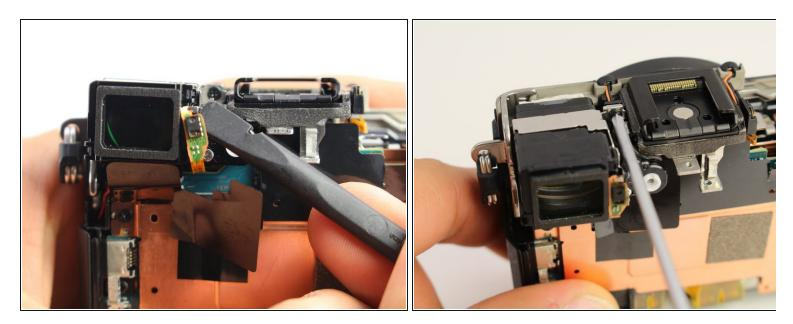
• Use the spudger to pry the light sensor off the side of the viewfinder.
