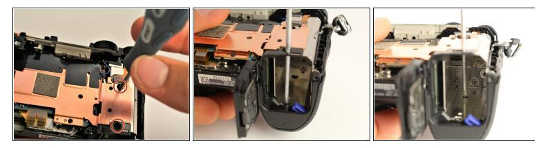
Insert a long, thin JIS 00 screwdriver through the two holes and into the battery compartment; remove the two 5mm JIS 00 screws inside it.
