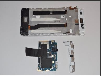
Carefully grip the motherboard and gently lift and remove it from the internal device casing.
