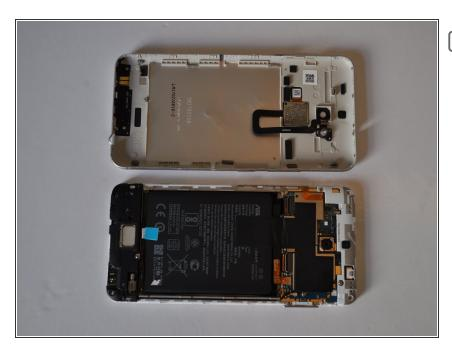
Once the original cover has been removed, apply the new cover to the back of the phone with careful pressure.
