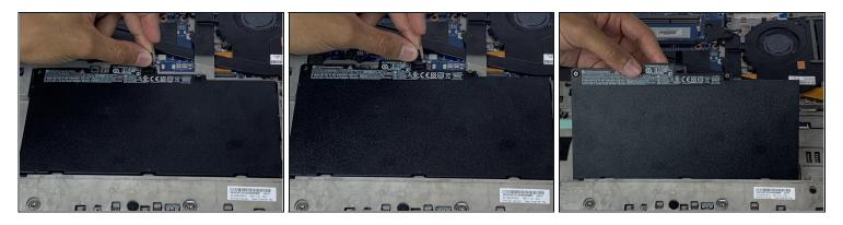
• Lift and pull the flap located at the top of the battery to remove it.
