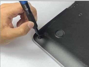
Use a Phillips #0 screwdriver to remove eleven 5.7mm screws.
