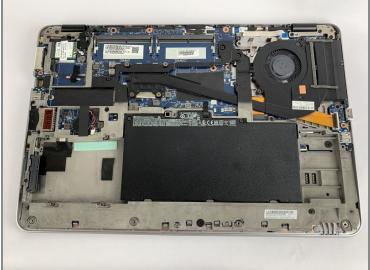
• Insert the iFixit opening pick underneath the plastic back of the laptop. Use force to pry the back off.
