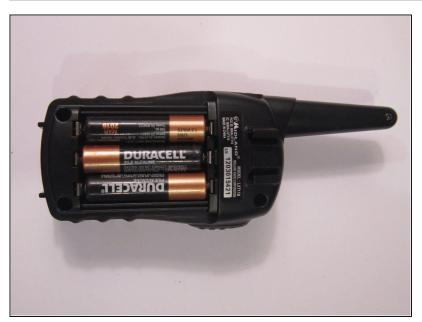
• Finally, once the cover is completely off, pry up the old batteries with your finger or a strong, skinny tool (i.e. spudger).
