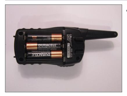
• Finally, once the cover is completely off, pry up the old batteries with your finger or a strong, skinny tool (i.e. spudger).
