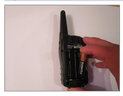
• Put the new batteries into their slots in the back case.
