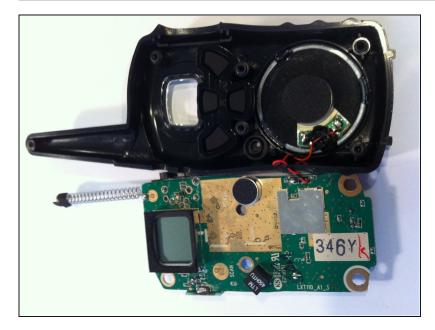
• Lay the circuit board down on the side, as you will not want it interfering with your work on the buttons!
