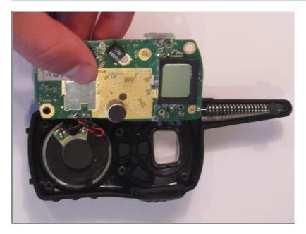
• Once the back case is already off, use your fingers to lift up the circuit board from the side opposite the antenna.
