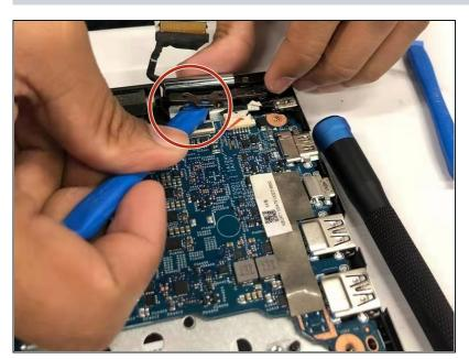
Use the plastic opening tool to pry the hinge up.
