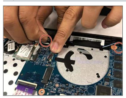
Detach the sensors on each side of the hinge from the motherboard.
