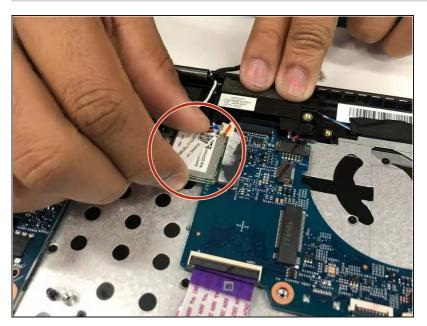
Remove the wireless LAN chip from the motherboard.
