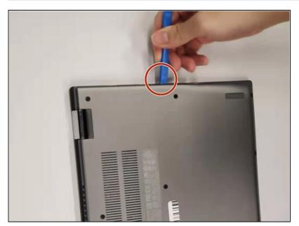
Use an opening tool to pry the back cover open.
