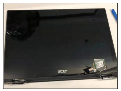
• Detach the screen assembly from the device.
